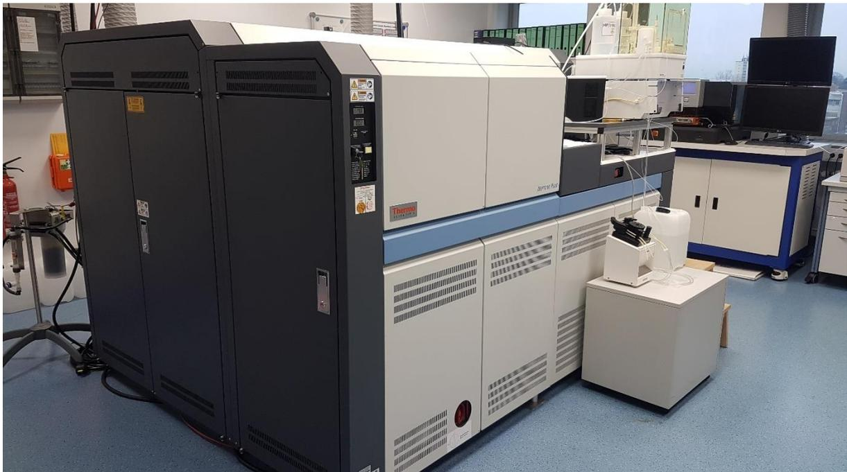
Abbildung 9: Thermo Fisher Scientific Neptune Plus Multicollector ICP-MS.
